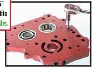
12. Install bearing retainer plate & screws using blue Loctite (242 or 243). Torque to 20-30 in-lbs.
