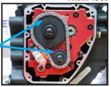
\* With the cam cover off during top end assembly you can easily rotate the engine and determine the stroke of the engine. This is a simple and precise way to determine which cylinder is on TDCC. \*
