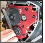
Use a straight edge to align cam drive sprockets. Alternate size spacers can be used to move rear cam sprocket in & out as needed.
