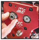
21. Using a sprocket locking tool install the sprocket retention hardware. Apply a small amount of moly lube to the under head flange of the bolts & Loctite 263 (Red) to the threads. Both bolts should be initially torqued to 15 ft/lbs. & then loosened one full rotation. Final torque the pinion shaft bolt to 24 ft/lbs. & the rear sprocket bolt to 34 ft/lbs.
