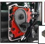
Use the proper sprocket locking tool & install the sprocket bolts using red Loctite. Final torque cam bolt to 34 ft/ lbs & crankshaft bolt to 24 ft/lbs.
