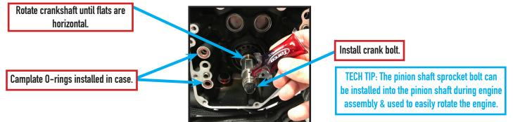
18. Install camplate & oil pump into cam chest as an assembly. As the assembly slides onto the crankshaft use your left thumb to press inward on the lower section of the oil pump & your right hand to guide the camplate at the same time. The assembly may need to be rocked to help guide the pump gears into place. If assembly doesn't install all the way, most likely the pressure gear flats are not lined with crank, or you may have a pinched o-ring.
