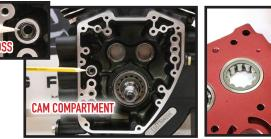
If installing the 1/16" boss plug, apply Loctite & torque to 55–60 in/lbs.
