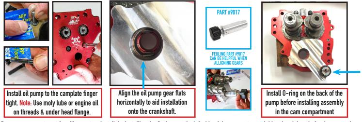
17. Prep cam compartment for oiling system install, by installing the O-rings on the left side of the compartment, lubing the pinion shaft & inner cam bearings. Install pinion sprocket bolt into the pinion shaft & rotate the engine until the flats are horizontal to match the oil pump gears.
