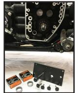
7. Wash, clean, & inspect the new FEULING components. Verify that all threaded holes around the profile are plugged & the pressure relief valve, spring & roll pin are installed. All Feuling camplates come with the pressure relief valve pre-set & tested from the factory.
