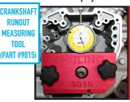
Crank runout under 0.005" Ideal is under 0.003". Including bearing play.
