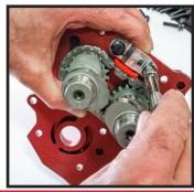
Torque fasteners to 120 in/lbs using moly lube on under head flange & threads.
