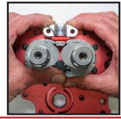
Install tensioner pad & housing square to the chain. Verify the pad moves up & down.
