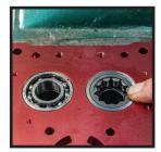
Chain drive roller bearing goes in the rear cam bore.
