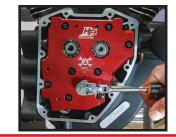
Rotate the engine 4–5 times to allign the camplate then tighten camplate bolts to 10 in/lbs.
