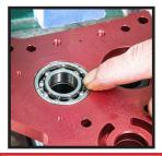
Ball bearing goes in the front cam bore.
