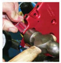
with Feuling's camplate pressure test tool #9010. We recommend pressure testing the camplate anytime it is out of the engine. It is important to test the camplate prior to disassembling the relief valve so you know how it is currently performing. The Feuling tool provides an ideal workstation for servicing the camplate.
