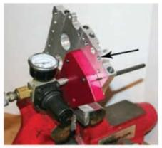
The arrow indicates the camplate oil port where you can feel for air leakage.
