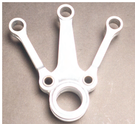
The conrod design for the W3 engine was based on that of ones used in radial aero engines
