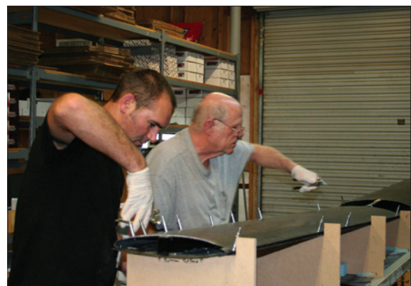
Luke Leatherman (left) and Gene Sheehan (right) working on the carbon fibre wings of the Feuling entry for the Green Flight Challenge
