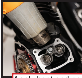
Apply heat and penetrating lubricant to the factory lifter cuff bolts.
