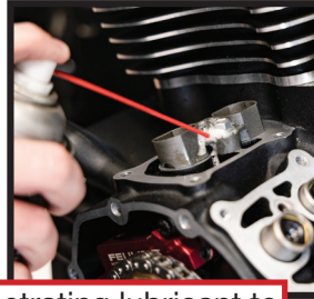
Apply heat and penetrating lubricant to the factory lifter cuff bolts.
