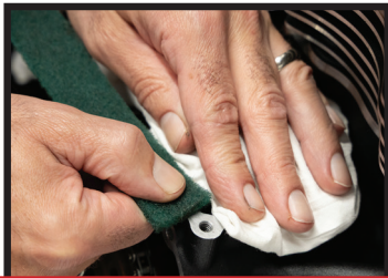
Cover lifter bores and passages when cleaning to prevent debris from falling inside.
