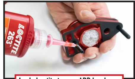
Apply Loctite to new ARP hardware
