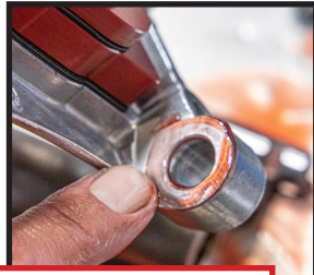
Lube rocker shafts & rocker arm support thrusting surfaces.
