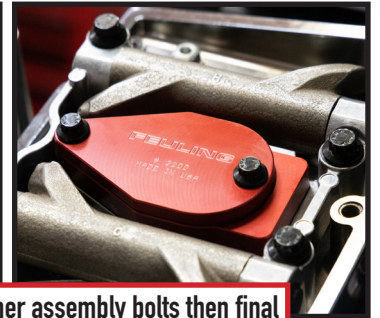
Apply Loctite to new ARP hardware
