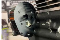
6.) Install oil filter adapter cover plate, install 3 allen (1/8" Allen), use loctite
