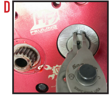
D Install front cam .100" thick thrust washer & retaining clip. Install clip with sharp ID edge outward.
