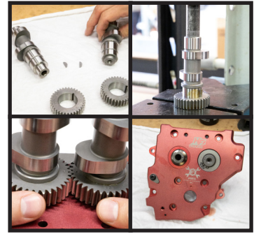
D Install front cam .100" thick thrust washer & retaining clip. Install clip with sharp ID edge outward.
