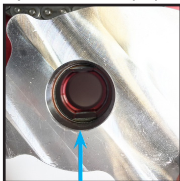
Align the oil pump gear flats horizontally to aid installation onto the crankshaft.
