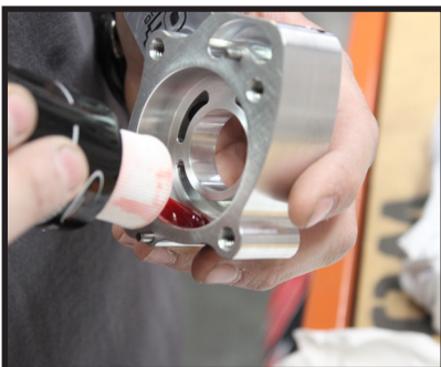
Apply assembly lube to the inside of the pump housings.
