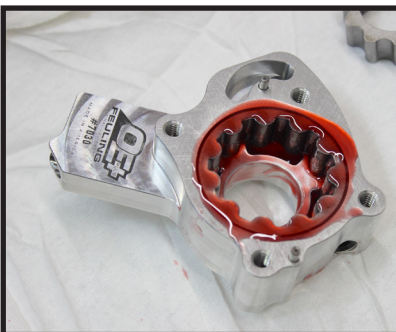
Lubricate the inner & outer gears of the oil pump.
