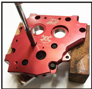
Install oil pump to the camplate finger tight. Note: use moly lube or engine oil on the fasteners.
