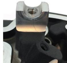
**HELP PREVENT M-EIGHT CYLINDER HEAD CRACKING!**
