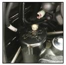
**OPTION 2.)** Quick disconnect fitting with rubber hose and filter element. This option will run any excessive oil misting/residue through the line and into the filter element. However this option does requires disconnecting the fitting in order to check the oil.
