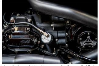
For option 2, we recommend routing the breather line along the transmission side cover using the supplied P clamp on the top left trans side plate bolt. Cleanly loop line up behind the battery box, under the seat, back down the right side frame rail and tuck the filter element up under the right side frame rail by oil pan.
