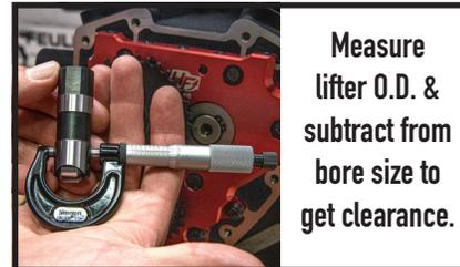
Measure lifter O.D. & subtract from bore size to get clearance.
