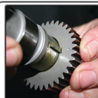
Line up gear with camshaft
