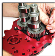
Install bearing retainer plate using loctite
