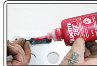
Apply Loctite to block off plate bolts
