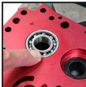
Ball bearing goes in the front cam bore.
