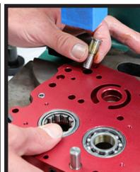
GEAR DRIVE NOTE: If running gear drive, do not install chain tensioner pins or chain guide tower.
