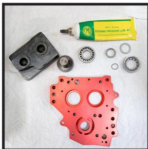
Press the bearings into the camplate using the proper press tools & lube, verify bearings are pressed square & flush with the camplate.
