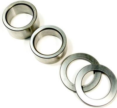
***Twin Cam Engine Crankshaft bearing race kits for A and B model engines. Kits includes right and left side crankshaft races with the left side thrust washers. These Feuling press on races have a precision ground outer diameter finish and are designed to be true to size producing the correct OD after proper press on installation***
