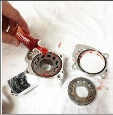
Clean and lube the oil pump and gears
