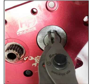
Install 0.100" thick thrust washer and retaining ring on front camshaft. Note the retaining ring installs with taper/bevel ID towards the camplate and the square ID towards the outside of the cam
