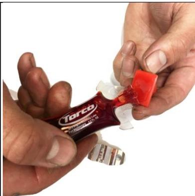
Lube tensioner pads, chains and inner bore of housings
