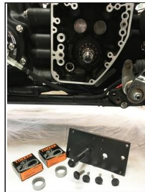
Install new inner cam bearings using the correct tools and press lube
