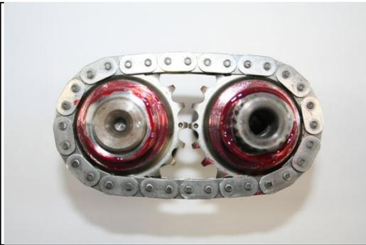
Picture showcases '07-'17 cams and or conversion camshafts with inner cam chain installed and timing marks lined up. Make sure chain is free of burrs and well lubed.
