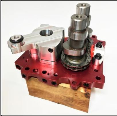
Assemble camplate, cams, inner tensioner and oil pump on the bench as a complete assembly. Oil pump should be finger tight, scavenge port O-ring should be installed on back of pump and well lubed.
