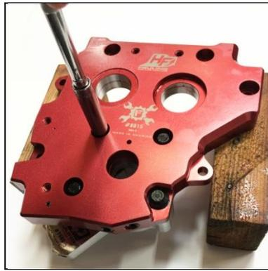
Install oil pump finger tight, do not use loctite on oil pump or camplate bolts, use moly lube or engine oil. Note we have the camplate supported by wood blocks to ease install of pump
