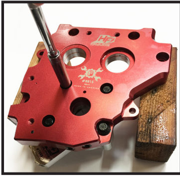
Install oil pump to the camplate finger tight. Note: use moly lube or engine oil on the fasteners.
