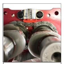
Make sure tensioner pad is square to the chain and the pad moves up and down.
