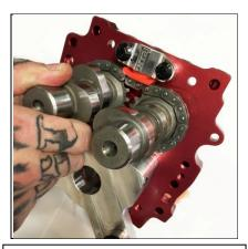
Rotate cams and verify the assembly rotates freely and the tensioner pad is true and not cocked.
