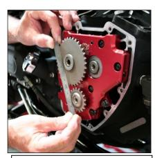
Align sprockets using a straight edge to verify sprockets are in line. Use the selection of different thickness thrust washer to adjust cam sprocket to match crank sprocket.
