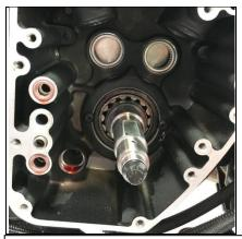
Rotate crankshaft so flats are horizontal. Install 2 camplate O-rings, put assembly lube on scavenge port hole of the case, O-rings, pinsionshaft and inner cam bearings.
