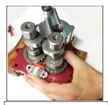
Install tensioner pads and housings squarely. Do not install 1 bolt then rotate tensioner housing into place as this can cock the pad.
