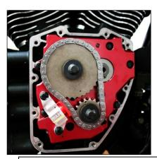
Install outer sprockets, cam and crank bolt and outer tensioner, use assembly lube on tensioner pad. Verify pad is square to chain
