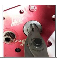
Install 0.100" thick thrust washer and retaining ring on front camshaft. Note the retaining ring installs with taper/bevel ID towards the camplate and the square ID towards the outside of the cam
