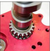
\*Always install new matching bearing race onto rear camshaft
