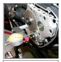
Engines that have premature tensioner pad wear should have the sprocket runout inspected. The sprocket registry on the crankshaft may need to be modified to true the sprocket.
