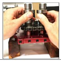
Feuling recommends supporting the camplate to ease installation and allow the camshafts to float freely. Wood blocks are used here. Properly lube camplate bores, cams, chain and always lead with the rear camshaft.
