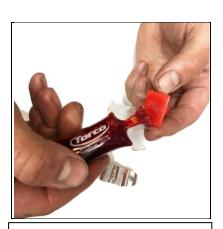
Lube tensioner pads, chains and inner bore of housings
