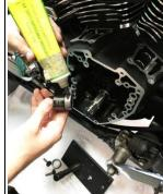
Install new inner cam bearings using the correct tools and press lube
