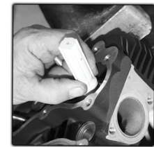
FEULING recommends the use a seal installer to prevent seal damage. Install spring, retainer & locks.
