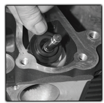
Pre-lube valves, install seat shims if needed, then install spring seats.
