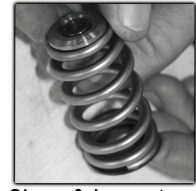
Clean & Inspect new springs & hardware
