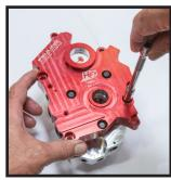
NOTE: DO NOT USE LOCTITE ON OIL PUMP OR CAMPLATE BOLTS, use moly lube paste, assembly lube or oil on bolt threads & underhead flange. Loctite will interfere with the stack up clearance of the oil pump & can cause sealing issues with camplate to engine case.
