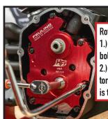
Rotate engine using the crank bolt.
