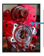
Use assembly lube on camplate bore, thrusting surfaces, camshaft & pinionshaft
