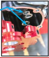
8. Install new 0-rings into engine case using assembly lube on 0-rings to aid in installation. Rotate crankshaft so flats are vertical.
