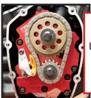
Step Torque cam & crank bolts first to 15 ft/lbs. loosen then re–step torque up to a final torque: Cam Bolt – 34 Ft/Lbs Crank Bolt – 24 Ft/Lbs
