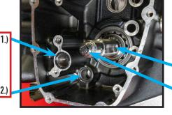
Install crank bolt then rotate crankshaft so the flats are vertical.
