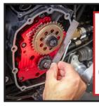
Check sprocket alignment with a straight edge.
