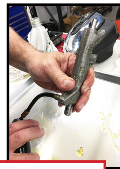
Manually pump up pushrods & rocker arms
