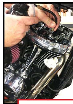
Manually pump up pushrods & rocker arms
