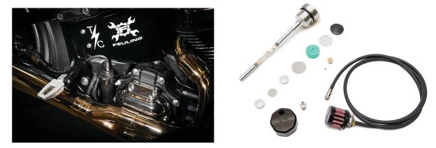
The FEULING® billet dipsticks vent/breathe excessive crank case pressure from the oil tank through a PCV style breather, consisting of an oil separator system, perforated disc, replaceable filter element and umbrella flapper valve. Feuling vented dipsticks screw into the factory oil fill spout as a stock replacement part. These breathing dipsticks remove unwanted build-up of blow by pressure in the oil tank.
