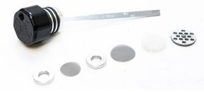
The FEULING® billet dipsticks vent/breathe excessive crank case pressure from the oil tank through a PCV style breather, consisting of an oil separator system, perforated disc, replaceable filter element and umbrella flapper valve. Feuling vented dipsticks fit into the factory oil fill spout as a stock replacement part. These breathing dipsticks remove unwanted build-up of blow by pressure in the oil tank.
