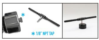
NOTE: THREADS ARE 1/8" NPT. DEPTH CAN BE ADJUSTED USING A 1/8" NPT TAP. TAKE CAUTION NOT TO GO TOO DEEP WHERE FITTING PUTS PRESSURE ON THE UMBRELLA VALVE. USE 1/8" NPT TAP IF DEEPER THREADS ARE DESIRED.
