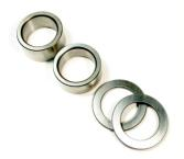
Twin Cam Engine Crankshaft bearing race kits for A and B model engines. Kits includes right and left side crankshaft races with the left side thrust washers. These Feuling press on races have a precision ground outer diameter finish and are designed to be true to size producing the correct OD after proper press on installation
