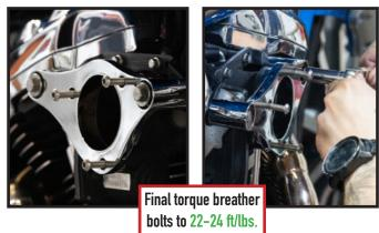
4. Apply red loctite to the velocity stack bolt threads. Attached velocity stack gasket and insert bolts through the bolt holes.
