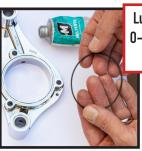
Lube backing plate 0-ring & install with 0-ring lube.
