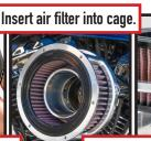
Line up metal tab on filter with cage post for best appearance.
