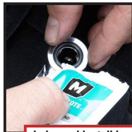
Lube and install inner and outer breather O-rings, use with O-ring lube.
