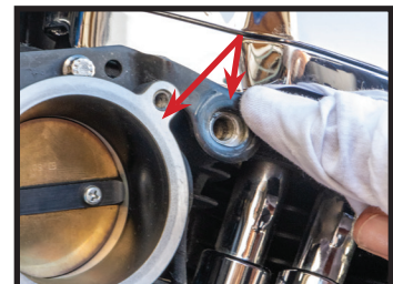
Clean breather holes & throttle body surfaces
