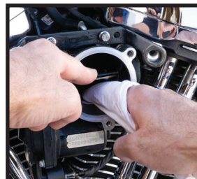
Clean throttle body & blade.
