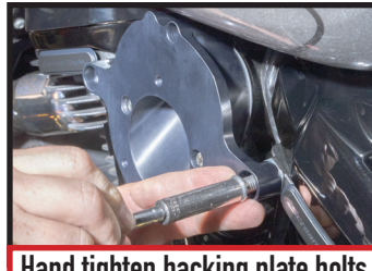
Hand tighten backing plate bolts
