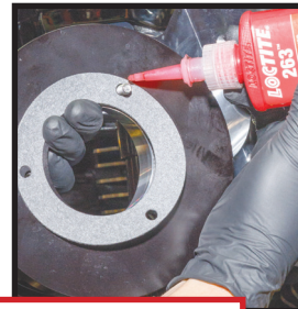
Install velocity stack and gasket. Apply red loctite to velocity stack bolts
