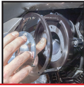
Install velocity stack and gasket. Apply red loctite to velocity stack bolts
