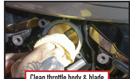
Clean throttle body & blade
