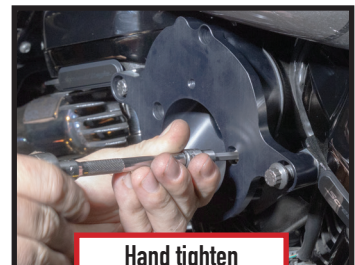
Insert velocity stack bolts to help center backing plate
