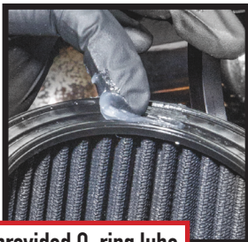
Lube air filter using provided O-ring lube
