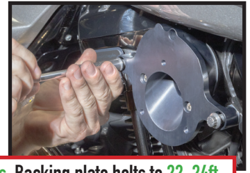
Torque throttle body bolts 72in lbs. Backing plate bolts to 22-24ft
