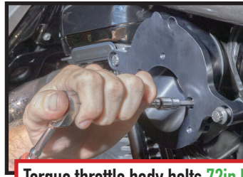
Torque throttle body bolts 72in lbs. Backing plate bolts to 22-24ft
