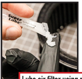
Lube air filter using provided O-ring lube
