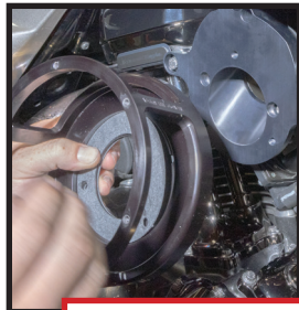
Install velocity stack and gasket. Apply red loctite to velocity stack bolts
