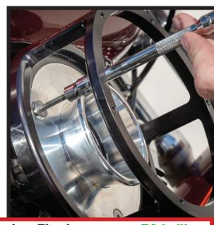
5. Lube both bases of the air filter to seal filter to cage & cover. Install filter gasket ring into cage, and insert air filter.
