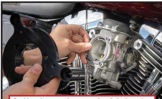
Backing plate to carburetor or throttle body gasket
