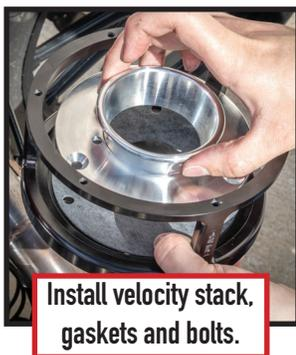
Install velocity stack, gaskets and bolts.
