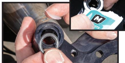
Lube and install inner and outer breather O-rings, use with O-ring lube.
