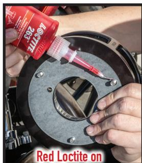
Red Loctite on bolt threads.
