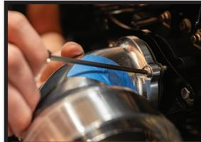
Use painters tape for protection when installing the upper right bolt
