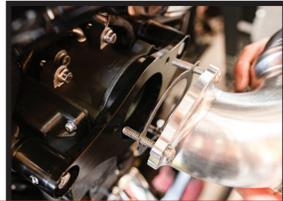
Insert the 3 bolts through the mounting holes and place the gasket onto assembly
