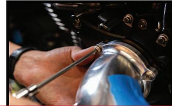
Tighten the other 2 bolts then final torque all 3 bolts to 72 in/lbs.
