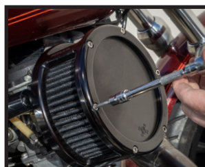
Final torque cover bolts to 30 in/lbs.
