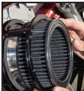
Install filter gasket ring into cage, Lube both filter bases with O-ring lube and install into
