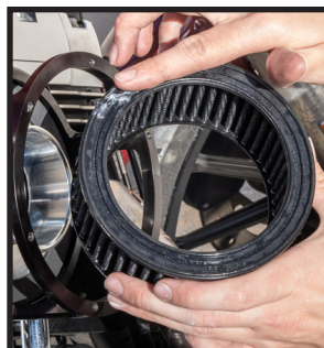
Install filter gasket ring into cage, Lube both filter bases with O-ring lube and install into
