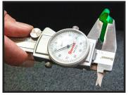
Measure thickness of clay after cycling engine.
