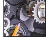
Verify camshaft lobe rotating clearance to engine case.
