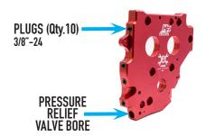
Verify camplate has all plugs (qty. 10) & the pressure relief valve, spring & roll pin are installed.
