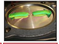
On high lift camshafts measure valve to piston clearance.
