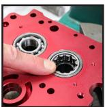
Chain drive roller bearing goes in the rear cam bore.
