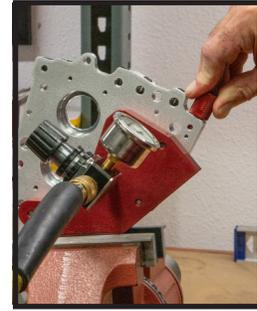
Use tool #9000 to hold down spring for easy removal of roll pin.
