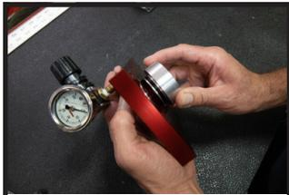
Install correct standoff plug for your model oil pump (oil or water cooled).
