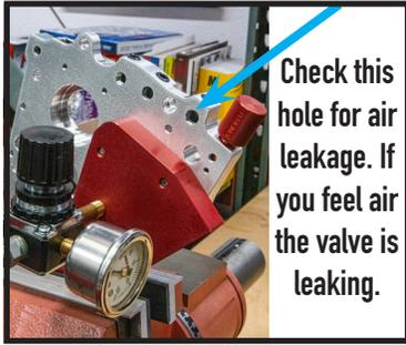
Check this hole for air leakage. If you feel air the valve is leaking.
