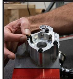
Use oil pump bolts to fasten pump housing to tool plate.
