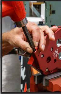
To re seat & seal valve use a hammer & punch to hit back of valve into seat, if needed use reamer (Part #9008) to cut a new seat in complete bore.
