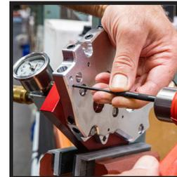
Use pin punch for final roll pin install.
