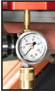
FEULING recommends: 50-65 PSI full pop off. Minimum 30 PSI re-seat & seal. The re seat & seal is important, any leakage at the valve will reduce oil psi
