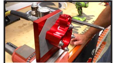
Pressure test oil pump housing.
