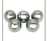
A set of precision ground steel balls to accurately measure lifter bore diameter and bore roundness.
