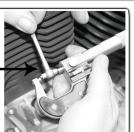
Measure lifter O.D. Subtract from Bore size to get clearance
